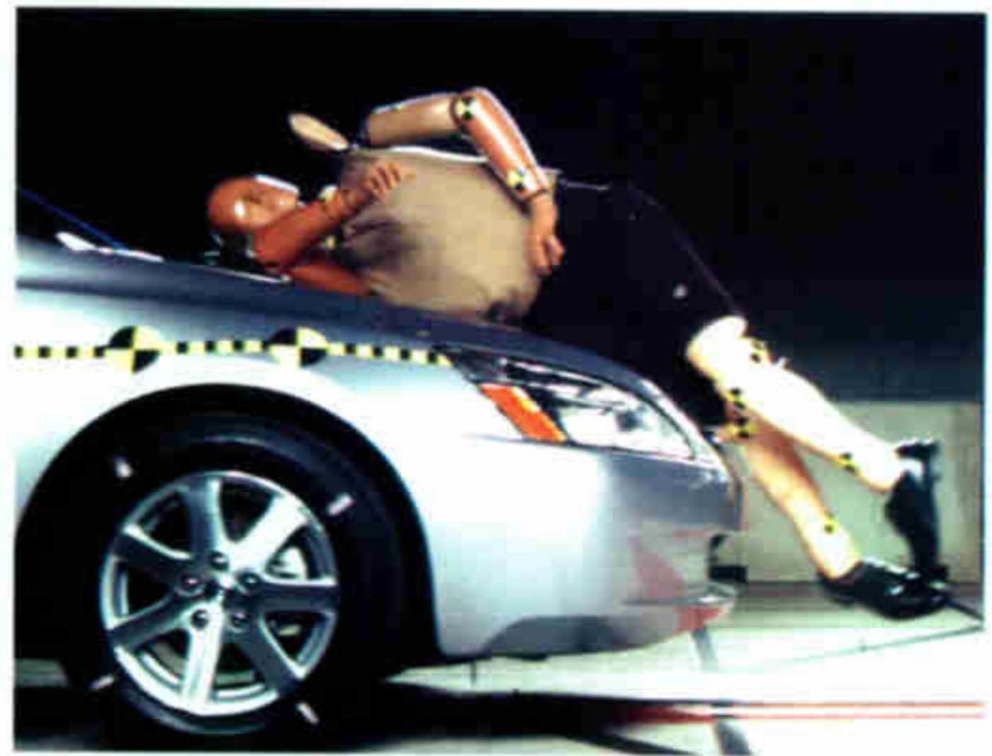
POLAR II has instruments that measure the level of injury throughout the body, including the head, neck, chest, abdomen and legs.
